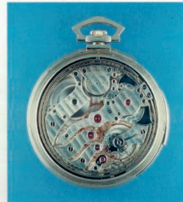
122b Rhodium-plated lever movement, 18''' SMQV calibre, extra-thin type, 29 jewels, bimetallic balance, Breguet balance-spring
